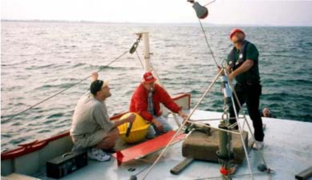
Figure 9. The RCM-9 current meter mounted in its tetrahedral frame on the deck of the RUSSELL B prior to deployment in Lake Ontario.
