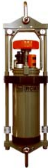
Figure 8. The Aanderaa RCM-9 acoustic doppler current meter. Photo courtesy of Aanderaa Instruments
